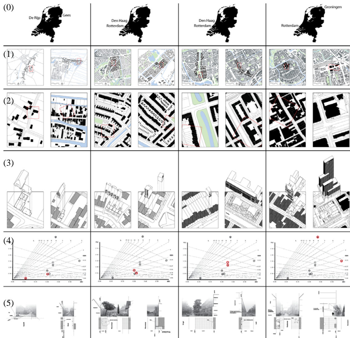
Figure 18. Overview of drawings on the five elements of the urban grammar. From top to bottom: location (0), city plan (1), parcelling plan and block type (2), building type and orientation (3), density (4), and public-private transition and street scene (5). From left to right: Gees, De Rijp, Rotterdam Vreewijk, The Hague Ypenburg, Rotterdam Heemraadssingel, The Hague Vaillantlaan, Groningen Oude Boteringstraat, Rotterdam Weena.
